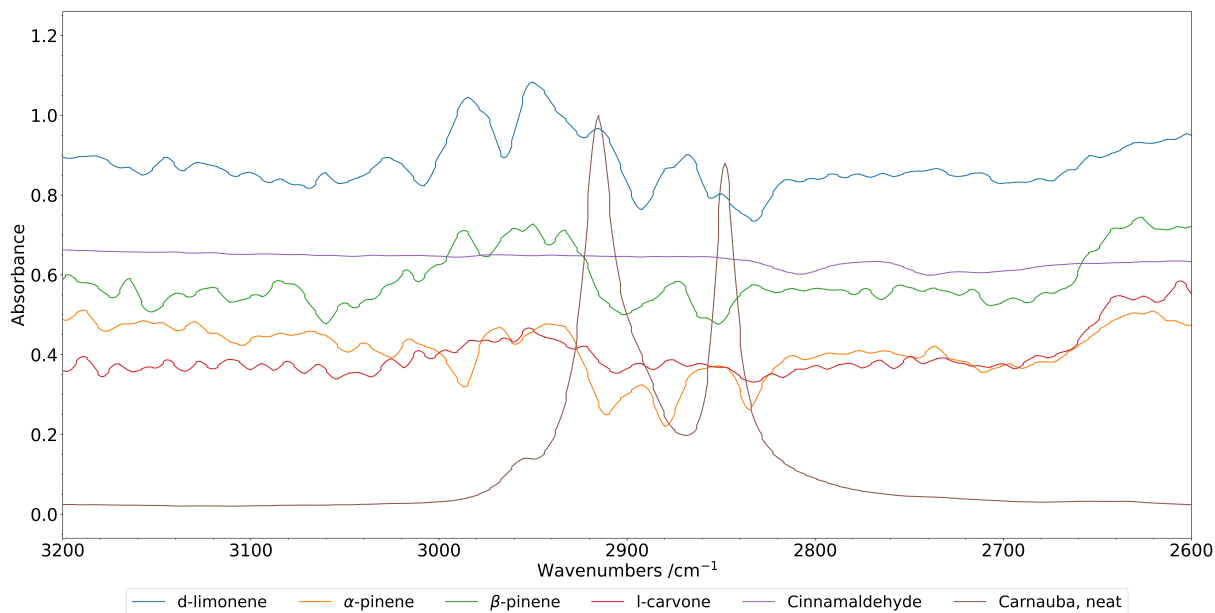
Figure 16. The difference spectra of each diffusant and carnauba wax compared to the neat spectrum of carnauba wax.
