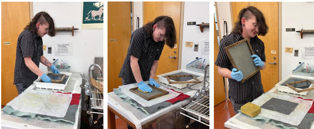
Figure 1: Daniel's papermaking process (pulling, couching, lifting)
