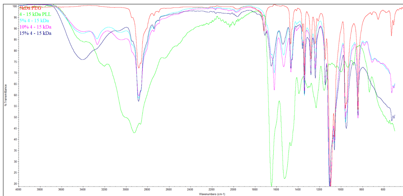
Figure 10. FTIR spectra of co-polymers resulted from 5, 10, and 15% PEGylation onto 4 – 15 kDa PLL.
