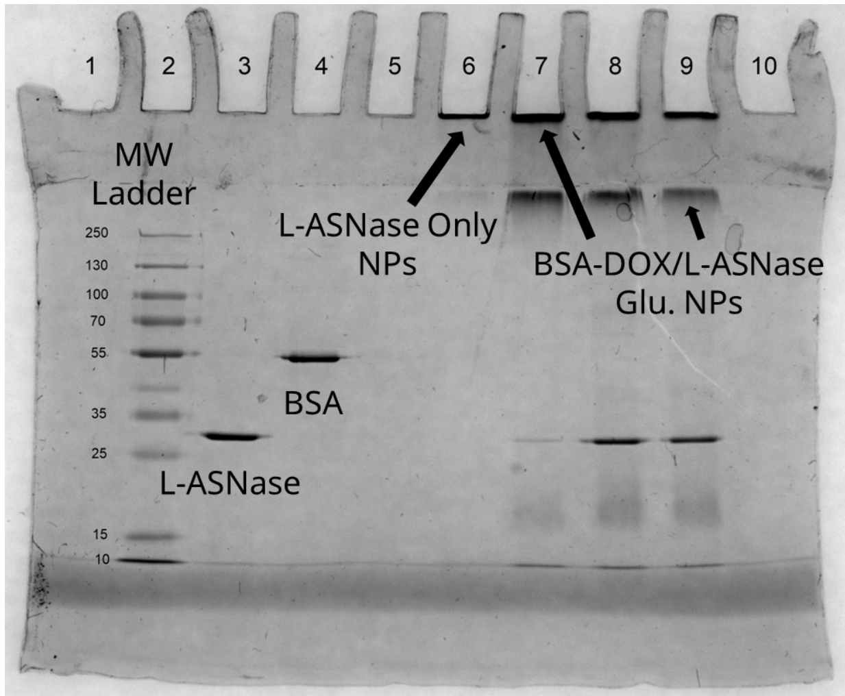
Figure 30 SDS-PAGE (12%) gel of L-ASNase/BSA-DOX Glu. NPs. Lane 2: Molecular Weight Ladder, Lane 3: 0.0885 mg/mL free L-ASNase, Lane 4: 0.0885 mg/mL free BSA, Lane 5: 0.0885 mg/mL free DOX, Lane 6: L-ASNase Only NPs, Lane 7: L-ASNase/BSA-DOX Glu. NPs 1, Lane 8: L-ASNase/BSA-DOX Glu. NPs 2, Lane 9: L-ASNase/BSA-DOX Glu. NPs 3.
