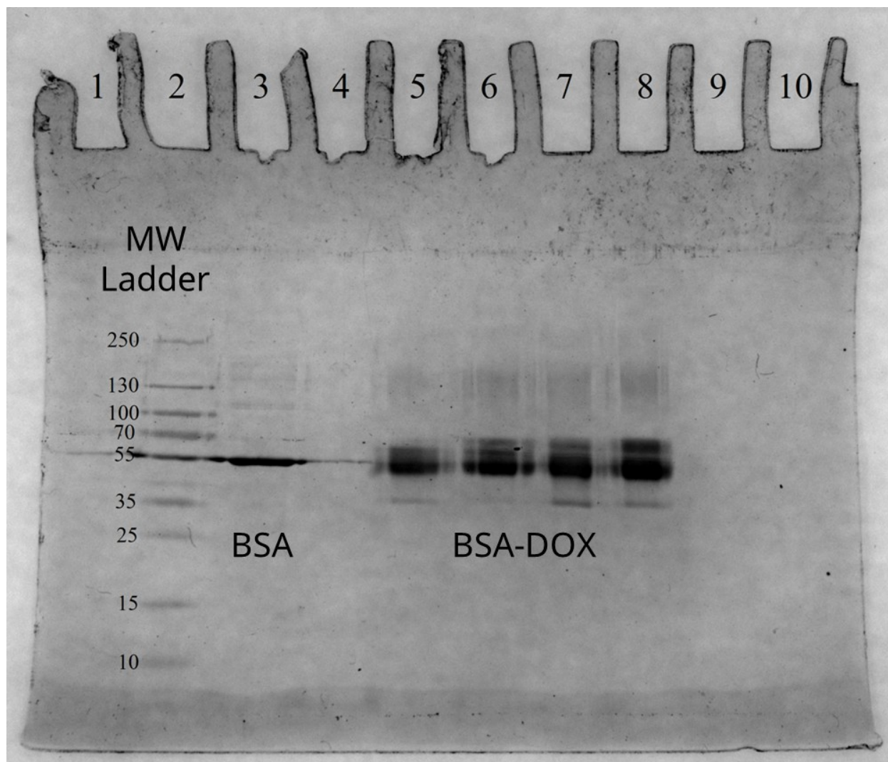
Figure 19 SDS-PAGE (12%) gel of BSA-DOX conjugates. Lane 2: Molecular Weight Ladder, Lane 3: 0.266 mg/mL free BSA, Lane 4: 0.266 mg/mL free DOX, Lane 5: 0.266 mg/mL BSA-DOX 1, Lane 6: 0.266 mg/mL BSA-DOX 2, Lane 7: 0.266 mg/mL BSA-DOX 3, Lane 8: 0.266 mg/mL BSA-DOX 4.
