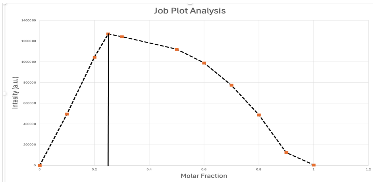
Graph 11b. A Job Plot analysis for PPi binding to ZnCl 2 L 1 (100uM) [excitation 440nm and emissions 591nm] at a 1:3 ratio in HEPES buffer (pH 7.4).
